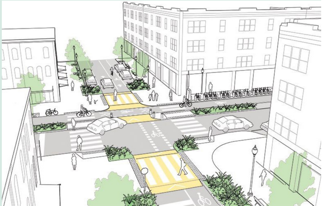
Rendering example of vertical deflection where raised crosswalks are implemented to calm traffic. Source: NACTO Urban Street Design Guide
